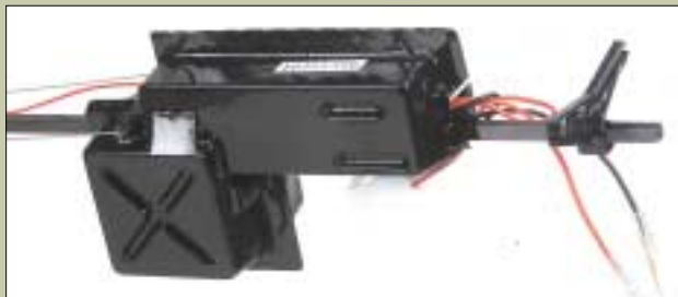
All onboard electronic equipment (servos, speed control and receiver) is already wired up and enclosed in this box, which comes mounted to the fuselage boom.
